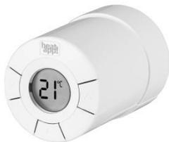
**heatapp! drive** is a radio component for the regulation of a radiator. **heatapp! drive** fit on all current brand valves with M30 x 1,5mm-connection or RA adapter. For valves with RA/V and RA/VL-valves we offer suitable adapters. Other adapters are available from the specialised trade.
